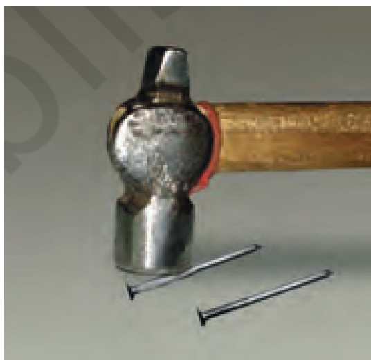
Fig. 2.4: Testing malleability of metal
