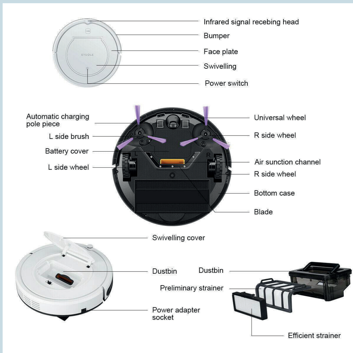
Fig. 3.2: Parts of a Robotic Vacuum Cleaner
