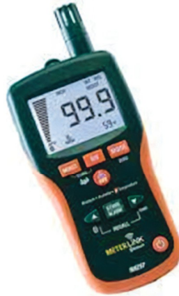
Figure 82: A picture of a Humidity Sensor
